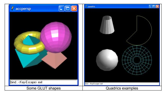
The shapes library consists of the C files (*teapot.c* for the teapot, *shapes.c* for all other shapes and the common header file *shapes.h*) and the Tcl file *tcloglShapes.tcl*.
